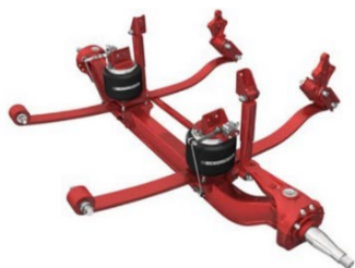
Original Manufacturer Equipment (Leaf/Air Primary Suspension)
