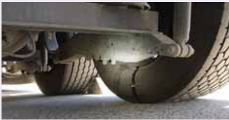
Inspectors identify an axle grease leak that could compromise a truck's brakes.
