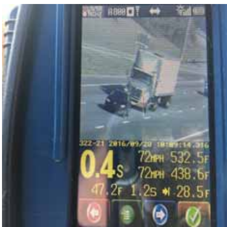
The LIDAR technology used by the Georgia Department of Public Safety's Motor Carrier Compliance Division has photographic and video capabilities built in.
