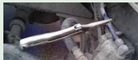
Air hose crimped with vice grips.
