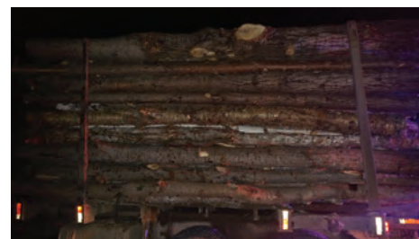
Longwood loaded lengthwise, no cargo securement used. Photo by Inspector Rod Dykeman, Nova Scotia, Canada.
