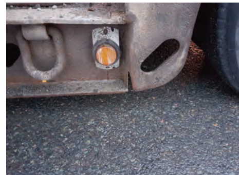
Low bed trailer separating at rear of deck. Photo by Inspector Alain Bilodeau, Nova Scotia, Canada.
