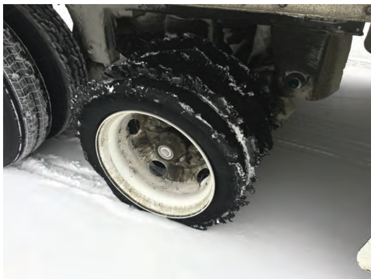
Dragged tires on a five-axle unit. Photo by Ofc. Brett Barteaux, Whitehorse Weigh Station, Yukon, Canada.
