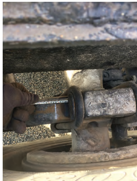
Loose U-bolts with axle shift. Photo by Inspector Lawrence Chard, Nova Scotia, Canada.
