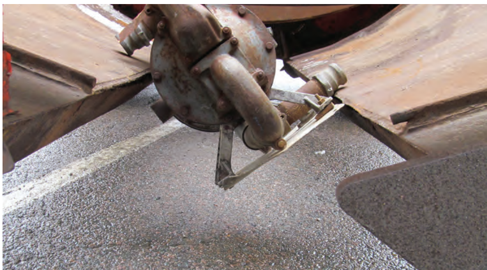
Belly dump trailer jaws open, causing insecure load. Photo by Inspector Ken Chisholm, Nova Scotia, Canada.
