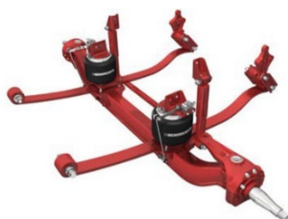
Original Manufacturer Equipment (Leaf/Air Primary Suspension)
