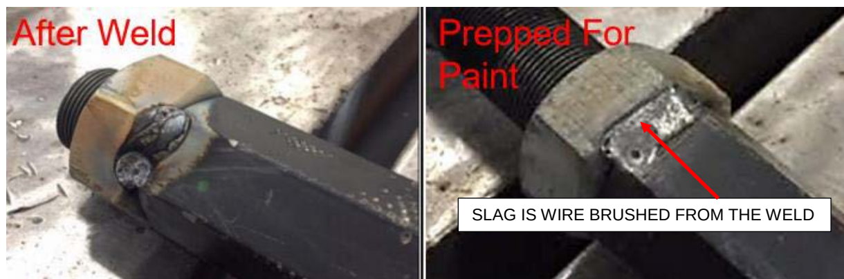
Figure 3: Drag Link Assembly with Welded Remedy Completed
