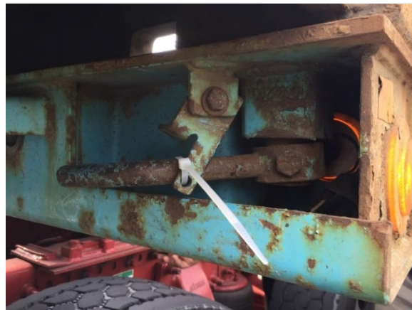
Figure 4: Use of Additional Tie-wrap
