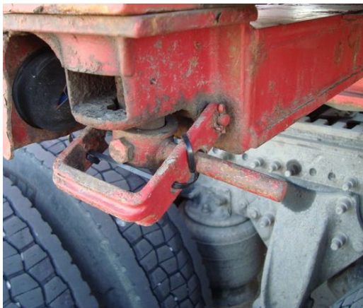
Figure 4: Use of Additional Tie-wrap
