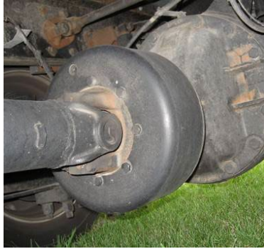
Example of a driveline type and wheel type parking brake
