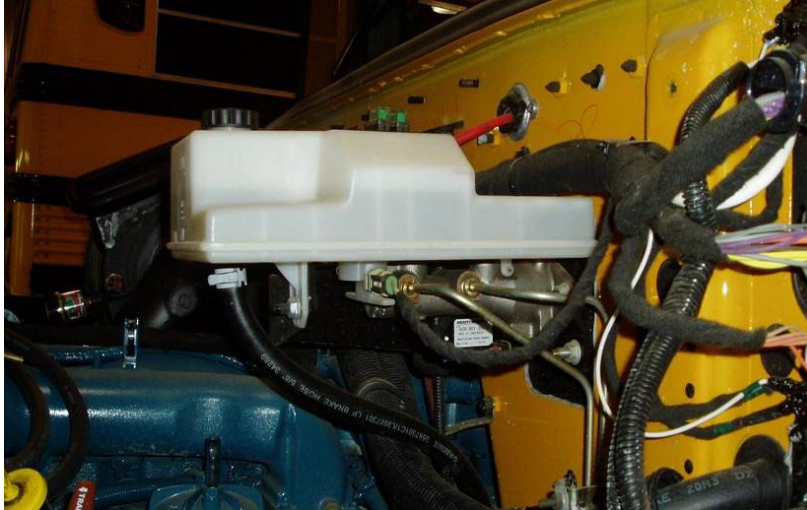
This is the firewall-mounted master cylinder.
