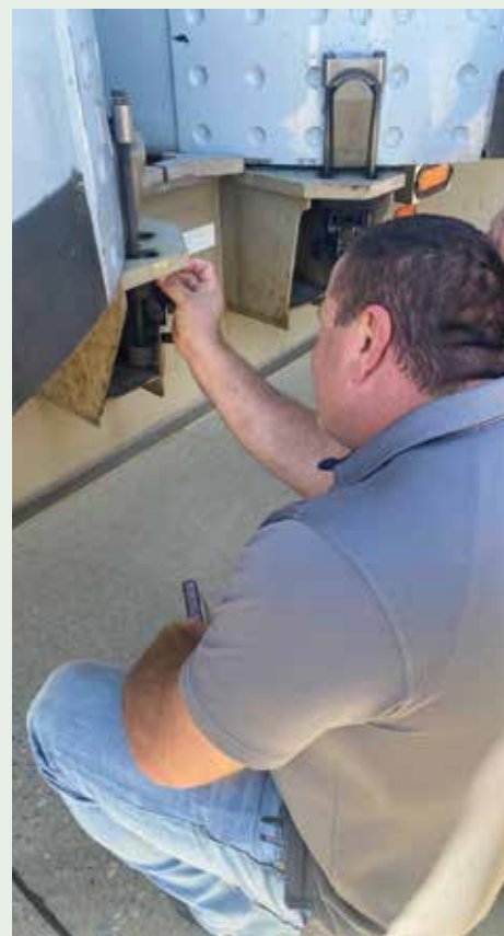
Kansas Highway Patrol Tpr. David Bales uses the go/no-go gauge on the securement device.
