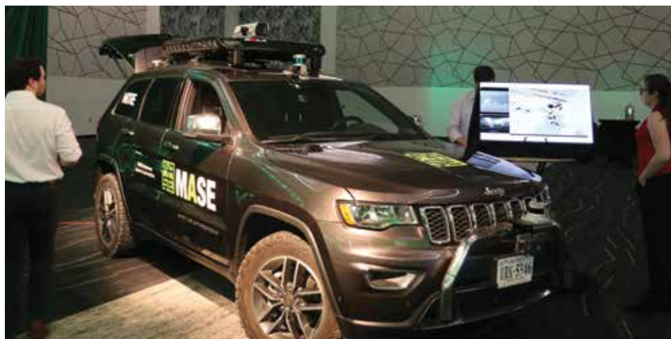
The conference included a DART. The Jeep Grand Cherokee has integrated drive-by-wire, computing, localization, perception and power electronics and is used for research purposes by MITRE.
