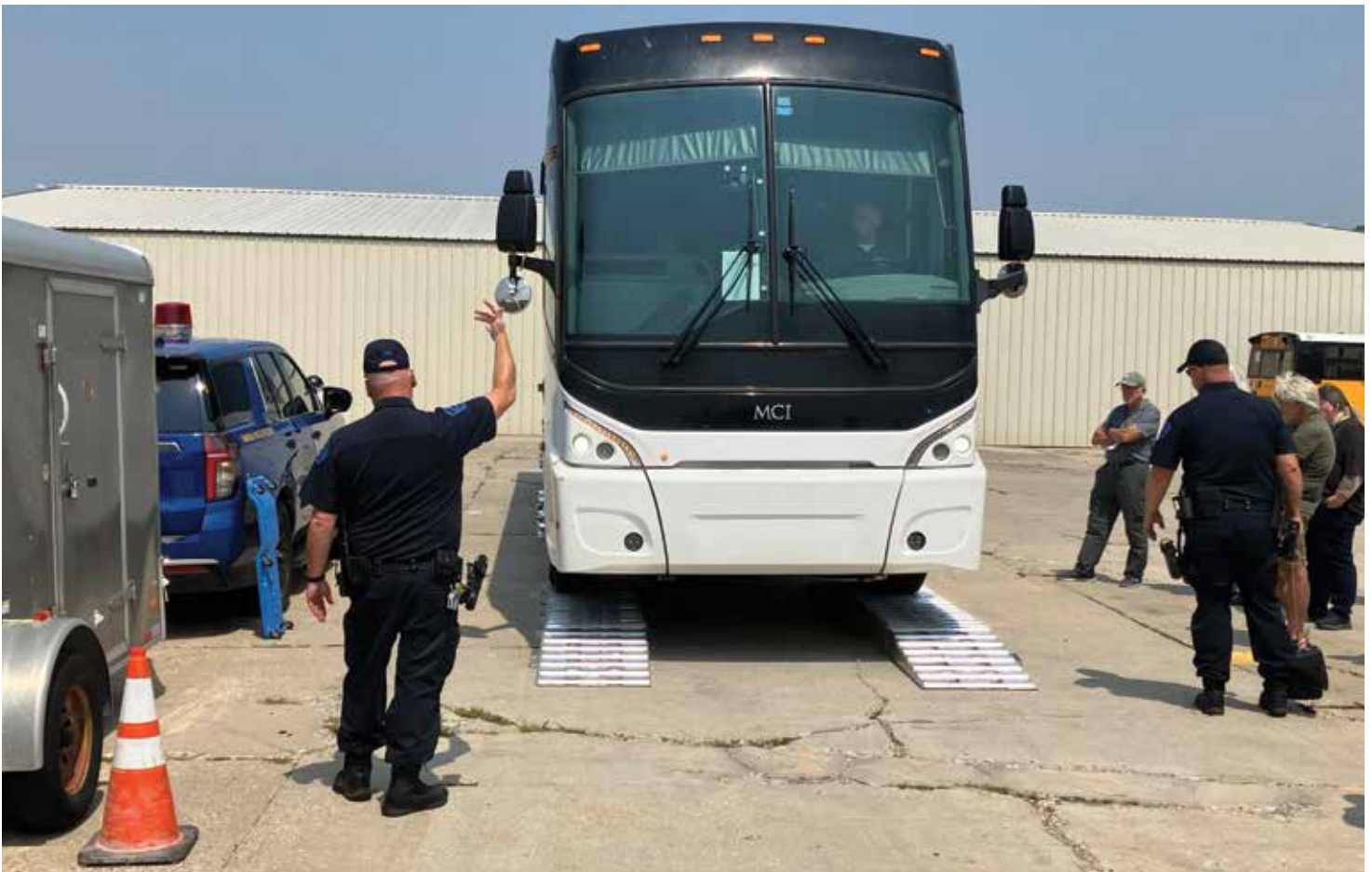
Sgt. Brian Ball and Ofc. Doug Dawdy demonstrate how to position a motorcoach on portable ramps for a Level I Inspection, assisted by Dean Trailways Trainer Ron Bosely behind the wheel.
