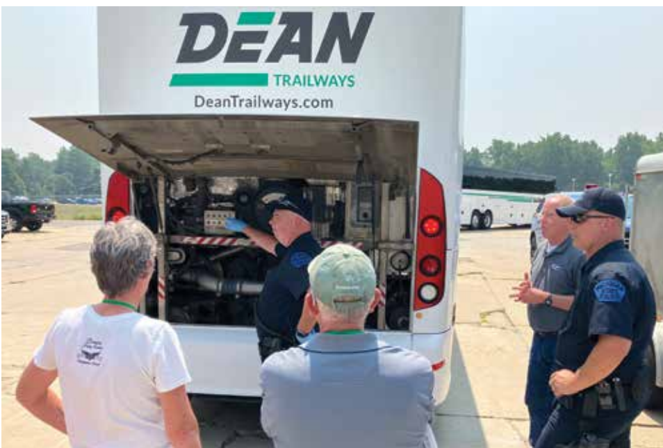
Sgt. Ball and Ofc. Dawdy walk attendees through the procedures for inspecting the engine compartment during a Level I Motorcoach Inspection.
