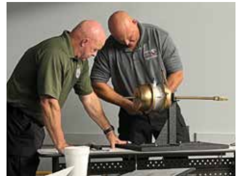
NCSHP Sgt. Michael Conley (left) and Master Tpr. Chelsey McGinnis (right) demonstrate changing a brake chamber diaphragm.
