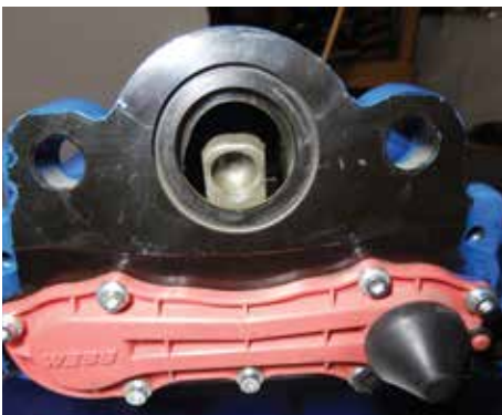
The location of the brake chamber mount.
