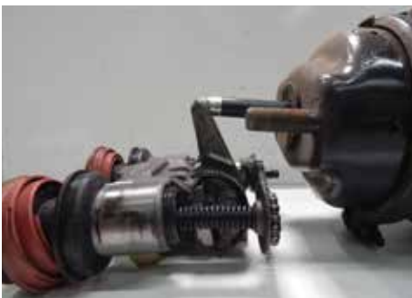
An internal view – note the lever, similar to a slack adjuster.
