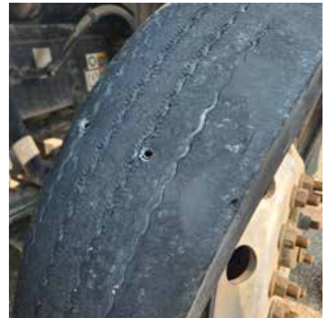
Larger, more rigid quills help to penetrate and deflate heavy truck tires.
