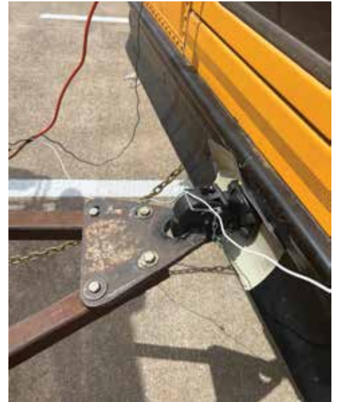
The front bus had a makeshift pintle hitch bolted only to the rear bumper.
