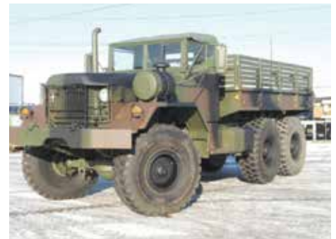
The M813A1 came out around 1980. It differed from the M54A2 in that the cable shut-off for fuel to the fuel pump was for emergency purposes, not daily use. I learned that one the hard way; after pulling out the handle and pushing it back in, the truck wouldn't start. It took me and a couple of mechanics half an hour to figure out why. The shut off had to be manually reset by hand at the fuel pump.
