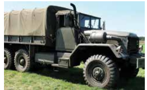
This is an example of one of the trucks I drove during my time in the U.S. Army. The M54A2 5-ton cargo truck was an older model from the Vietnam War era. The cargo cover was removed to make room for two 600-gallon pods, and reel unit with a single cylinder pump unit.
