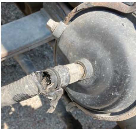
Hole in brake chamber hose.
