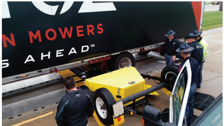
A performance-based brake tester is a machine that assesses the braking performance of a commercial motor vehicle.
