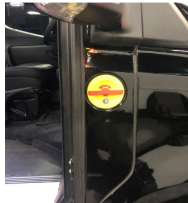
Exterior door release valve at the entrance door of a custom limousine.
