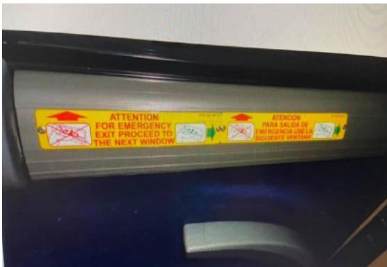
Pictograph and text clearly indicating this non-opening window is not an emergency exit and the location where the exit may be
